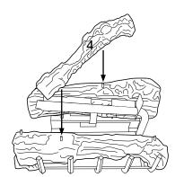
Figure 48 - Installing Log No. 4
